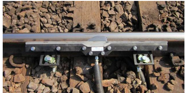
Figure 9: Wiping bar for TOR unit.
