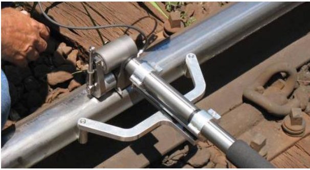
Figure 12: Rail Miniprof for rail wear monitoring.
