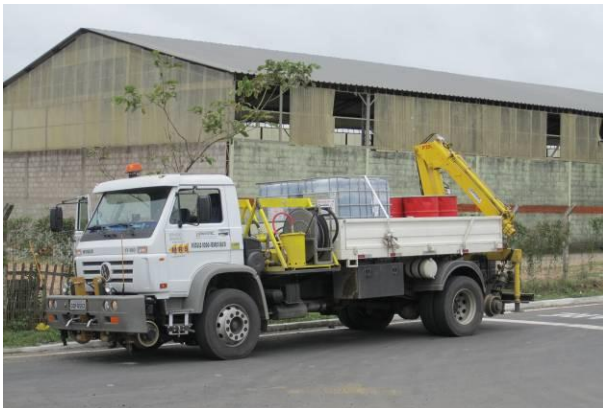
Figure 10: Hi-rail truck for filling and installation services.
