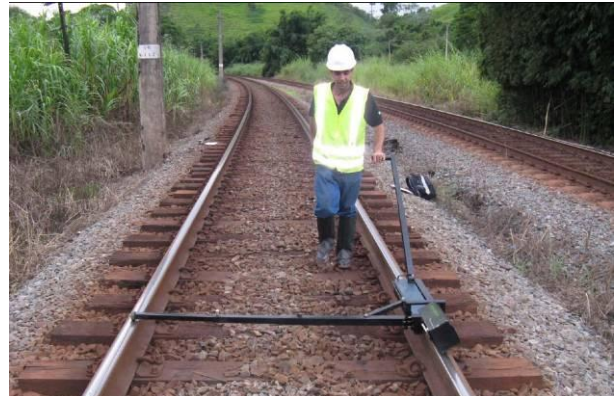
Figure 11: Measurement of COF using Tribometer.
