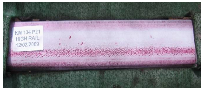
Figure 4 – Dye penetrant for rail surface evaluation
