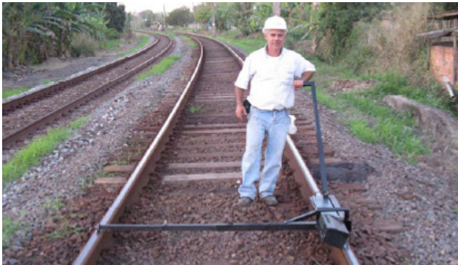
Figure 5 – Friction coefficient measurement on track using the push tribometer
